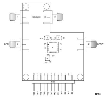
Figure 3. SKY65372-11 Evaluation Board Assembly Diagram
