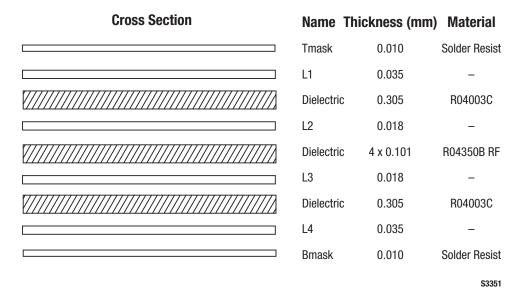
**Figure 5. Layer Detail Physical Characteristics**
